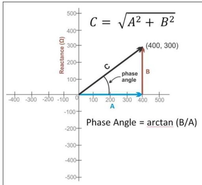
So, the impedance of your dream,  $Z = 50 + j0$  can also be written as  $Z = 50$  ohms with a 0-phase angle, or '50 ohms of purely resistive Impedance'.
